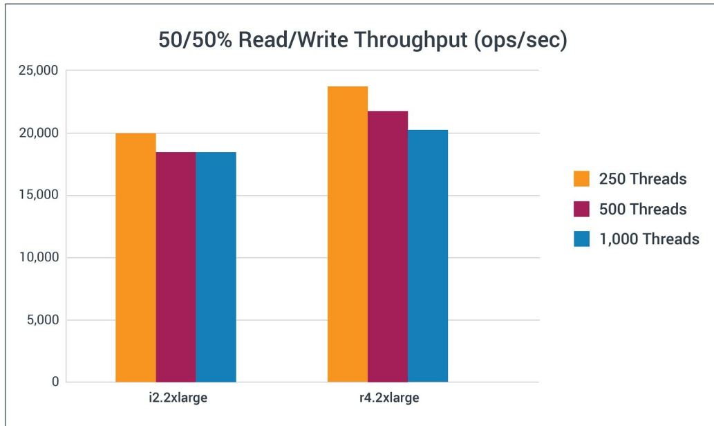
Figure 2: Throughput for i2.2xlarge and r4.2xlarge Instances
